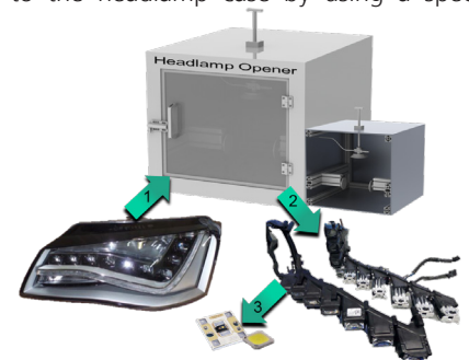
A new service process for faulty LEDs in LED headlamps using the 'headlamp opener'.
