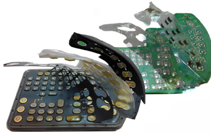
Fig. 1: Disassembly of the membrane keypad used heat to soften the glue and separate the membrane from the printed circuit board (PCB).
